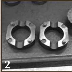
2 Install alignment pins/springs into driver holes
