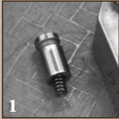
1 Place springs in hollow end of alignment pins
