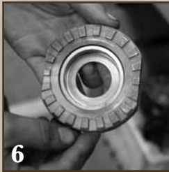
6 Install spacers into the center drivers
